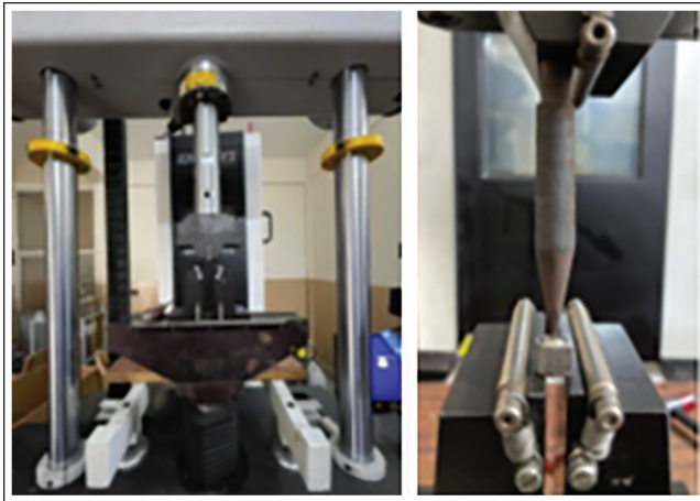
Figure 3. Universal Testing Machine and Samples Prepared for Push-out Test.
